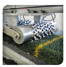
Our fully equipped test unit checks the installation of JUTAgrass® lawns according to the requirements of the FIFA Quality Programme.
