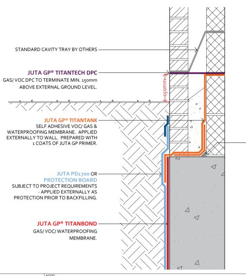
– ALL CORNERS TO BE REINFORCED WITH A MIN. 40mm CEMENT FILLET AND REINFORCING STRIP OF JUTA TITANTANK
