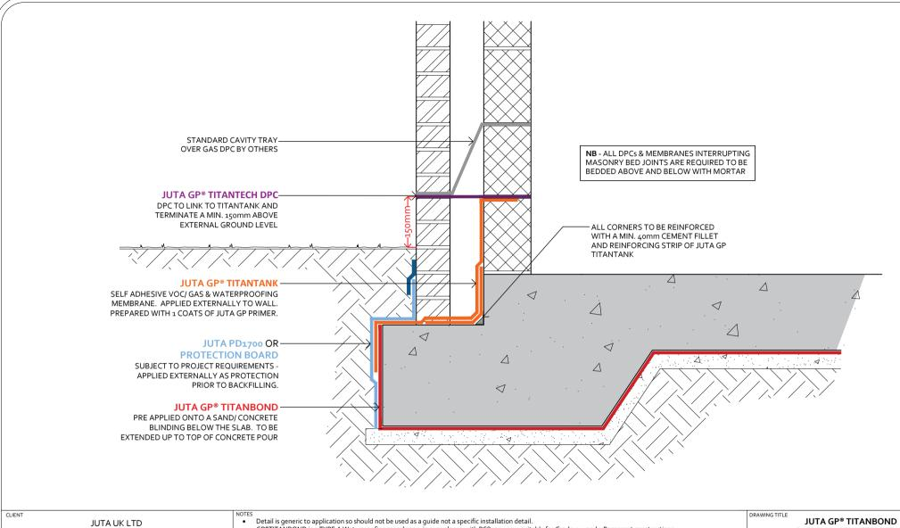
PROJECT GP® TITANBOND - Standard Details JUTA GP®TITANBOND is a TYPE A Waterproofing membrane, in accordance with BS8102:2009, suitable for Grade 1, 2 and 3 Basement constructions.
