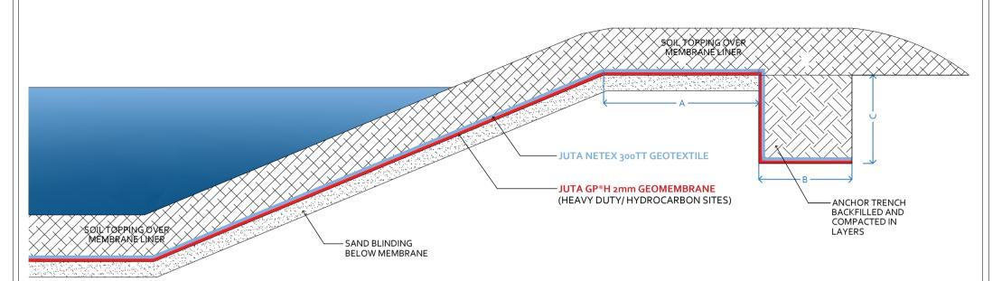
TYPICAL SWALE LINER DETAIL
