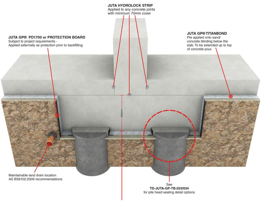
Pile caps less than 600mm likely to require fully wrapping (subject to project requirements) contact JUTA for further info
