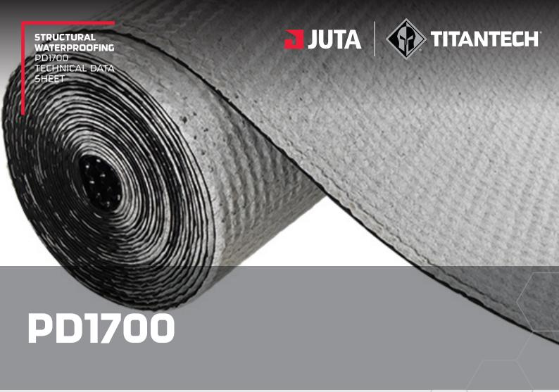
JUTA PD1700 include a high compressive strength Cuspate High Density Polyethylene (HDPE) Drainage core with a geotextile filter geotextile bonded to one side. Protection Drainage (PD) 1700 is designed as a high flow medium to alleviate hydrostatic pressure on below ground structures, as well as providing protection to the underlying membrane (gas/waterproofing).
