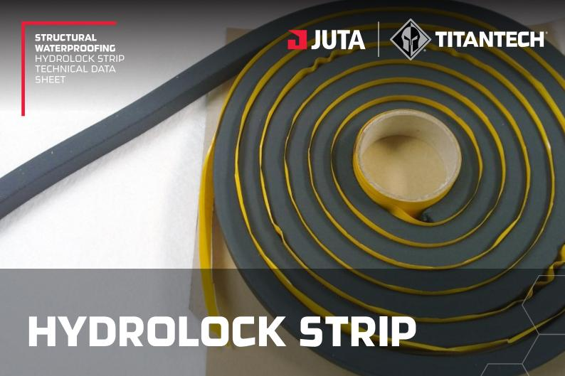
HYDROLOCK STRIP is a swellable bentonite joint sealing tape with crystallization additives. HYDROLOCK STRIP is used as a waterstop in concrete construction joints, and is tested and approved up to 7 bar water pressure.
