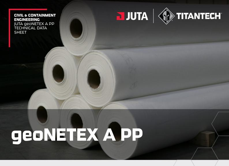
JUTA geoNETEX A PP (300 TT) is a nonwoven geotextile manufactured from UV stabilised, high tenacity, virgin polypropylene fibres that have been mechanically entangled to provide high strength, high extensibility, high loft and excellent abrasion characteristics.
